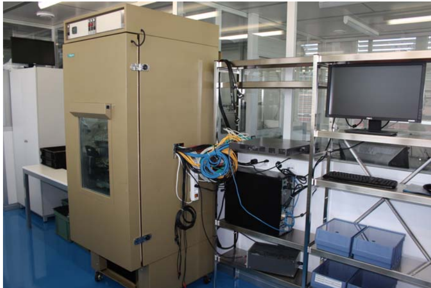
Image 18: Clima chamber for burn-in tests from -20 to +100°C
