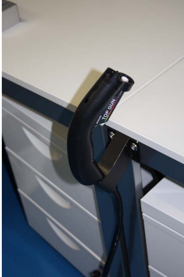
Image 15: Deionizing air gun for cleaning- and deionizing process
