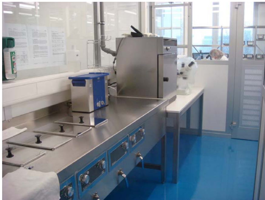
Image 2: 4 ultra sound units and the drying chamber
