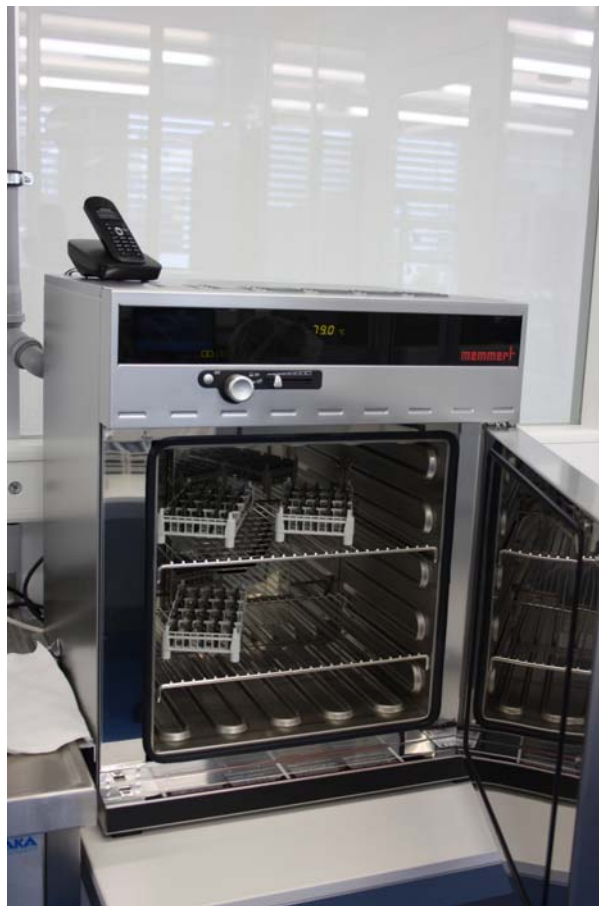
Image 6: Drying chamber from Mammert (Germany)
